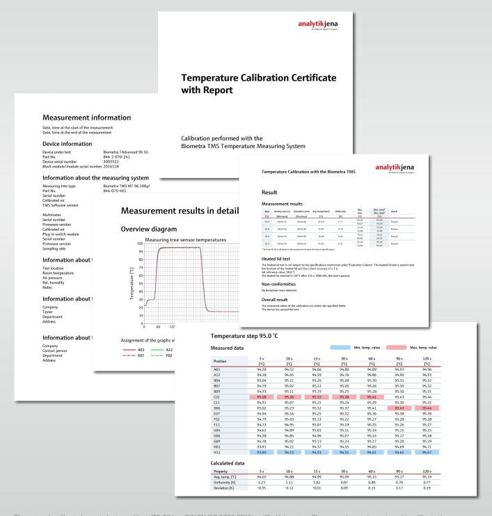
The system is calibrated so as to be traceable to ITS-90 by a DIN EN ISO 9001:2015 certified laboratory. The measuring equipment used to calibrate the measuring system is regularly calibrated according to DIN EN ISO 17025 in a DAkkS-certified laboratory and is traceable to national or international standards.
